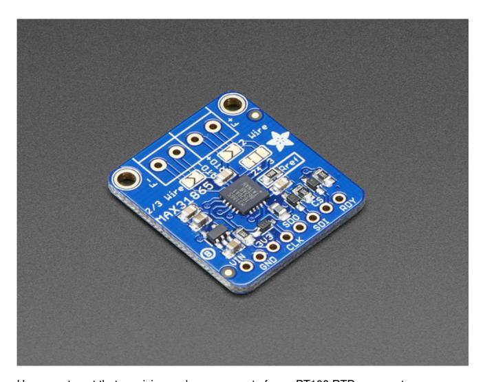
However, to get that precision and accuracy out of your PT100 RTD you must use an amplifier that is designed to read the low resistance. Better yet, have an amplifier that can automatically adjust and compensate for the resistance of the connecting wires. If you're looking for a great RTD sensor, today is your lucky day because we have a lovely Adafruit RTD Sensor Amplifier with the MAX31865 sensor.
