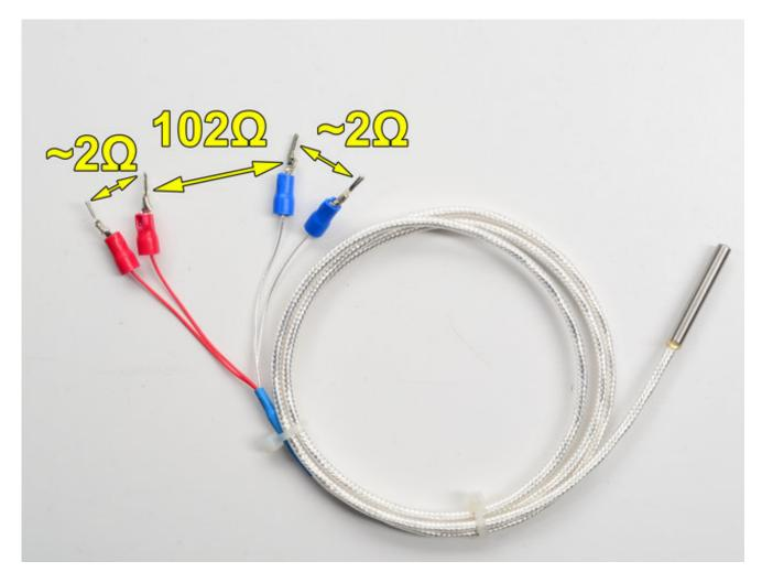
(Remember that the  $102\Omega$  will vary with temperature, but the  $2\Omega$  wires will not) When the amp measures this sensor, it will measure the resistance between one set of red and blue wires. It will then measure the resistances between the red wires and blue wires. Then divide those resistances by half - since there's two wires and we just want the resistance of one wire. The final result is  $102 - 1 - 1 = 100\Omega$
