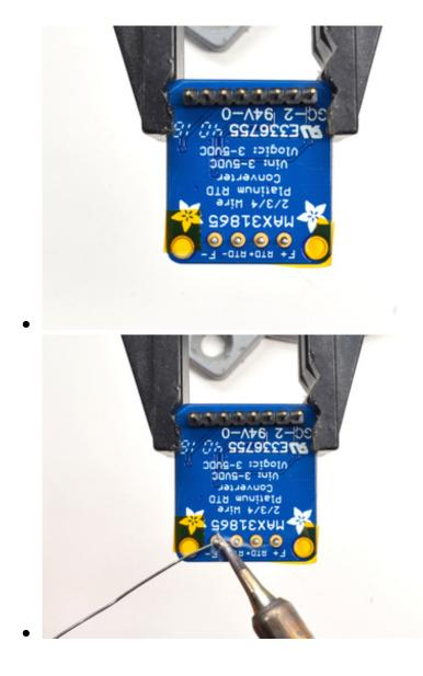
Solder in both pins of each terminal block. You can
