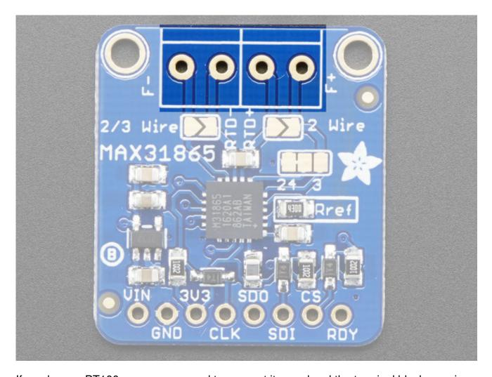
If you have a PT100 sensor, you need to connect it somehow! the terminal block area is where you can clamp down to the sensor wires.
