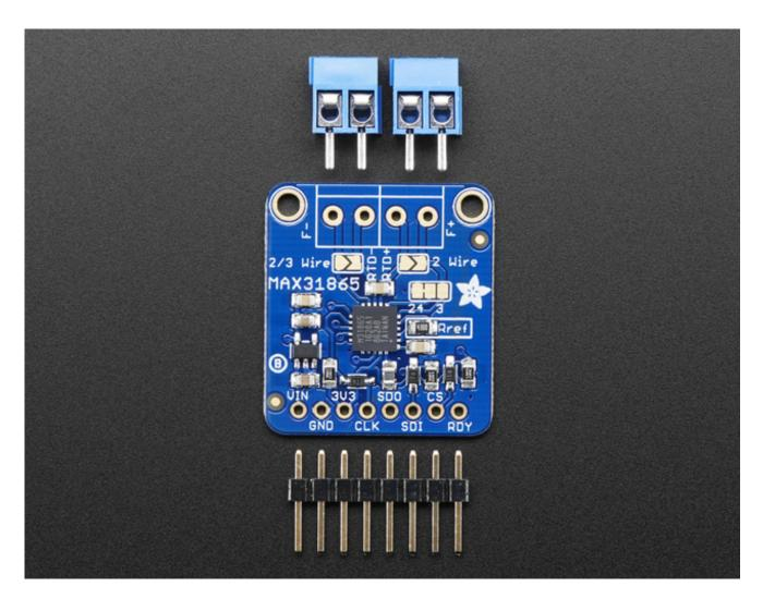
Each order comes with one assembled RTD amplifier breakout board. Also comes with two 2-pin terminal blocks (for connecting to the RTD sensor) and pin header (to plug into any breadboard or perfboard). **A required PT100 RTD is not included!** (But we stock them in the shop). Some soldering is required to solder the headers and terminal blocks to the breakout, but it's an easy task with soldering tools.
