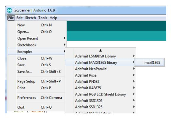
Upload to your Arduino and open up the serial console at 115200 baud to see a print out of the sensors data. The MAX31865 doesn't actually return the resistance it measures. Instead it returns the *ratio* between the resistance measured and the **Rref** reference resistor. For Adafruit breakouts, this is a 430 ohm 0.1% resistor. You can use that ratio to calculate the resistance and then determine the temperature
