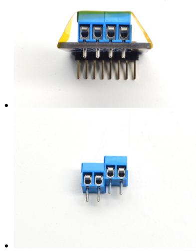
Next we will solder in the two 3.5mm terminal blocks used to connect power & the motor to the breakout board.
